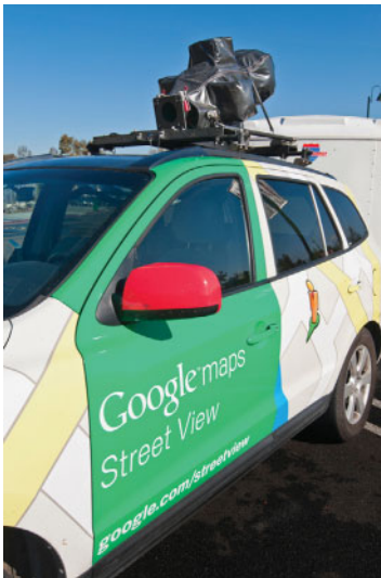
Figure 14.5 Google vehicle with camera attached to photograph images used in Street View maps.
