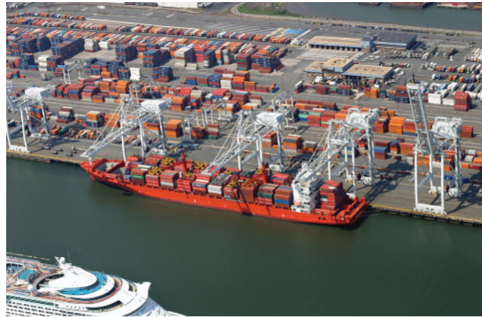
Figure 9.10 Examples of intermodal transportation ports. Container ships from around the world are unloaded in the Brooklyn, New York (left), and Bayonne, New Jersey (right), shipyards. Containers are tracked as they are loaded onto trucks or rail and transported across the country.
