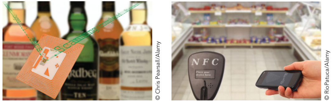
Figure 1.22 NFC technology relies on sensors or RFID chips. NFC is used for tracking wine and liquor to manage the supply chain efficiently. NFC smartphones are being integrated into payment systems in supermarkets so customers can pay for purchases without cash or credit cards.
