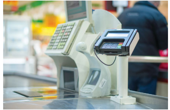
Figure 5.2 POS payment terminal. Malware-infected POS terminals caused Target’s data breach.
